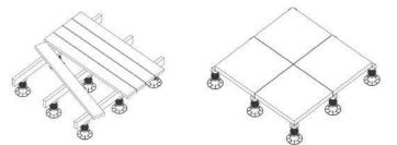
\*\*SKYJACK pedestals can be used with any size or shaped materials including deckingand concrete pavers. Simply remove spacer tabs and re-position in the holes that provide appropriate spacing
